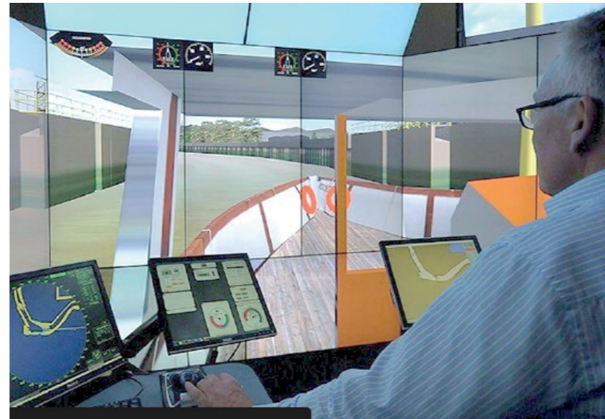
The project's BIM model was used to develop virtual navigation simulations for river users.
